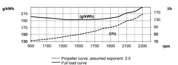
Test conditions Air temperature +25°C. Barometric pressure 100 kPa (750 mmHg). Humidity 30 %. Diesel fuel acc. to ECE R 24 Annex 6. Density of fuel 0.840 kg/dm². Viscosity of fuel 3.0 cSt at 40°C. Energy value 42700 kJ/kg. Power test code ISO 3046. Power and fuel values +/-3%.
