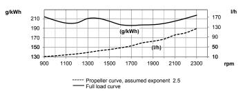
Test conditions Air temperature +25°C. Barometric pressure 100 kPa (750 mmHg). Humidity 30 %. Diesel fuel acc. to ECE R 24 Annex 6. Density of fuel 0.840 kg/dm³. Viscosity of fuel 3.0 cSt at 40°C. Energy value 42700 kJ/kg. Power test code ISO 3046. Power and fuel values +/-3%.
