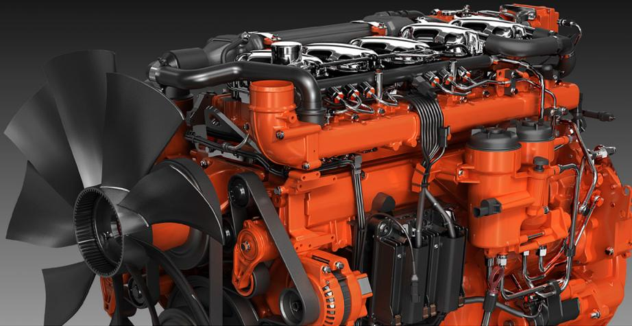
The industrial engines from Scania are based on a robust design with a strength optimised cylinder block containing wet cylinder liners that can easily be exchanged. Individual cylinder heads with 4 valves per cylinder promotes reparability and fuel economy.
