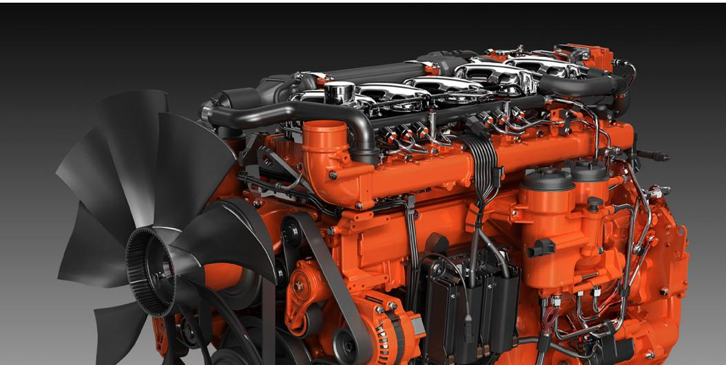
The industrial engines from Scania are based on a robust design with a strength optimised cylinder block containing wet cylinder liners that can easily be exchanged. Individual cylinder heads with 4 valves per cylinder promotes reparability and fuel economy.
