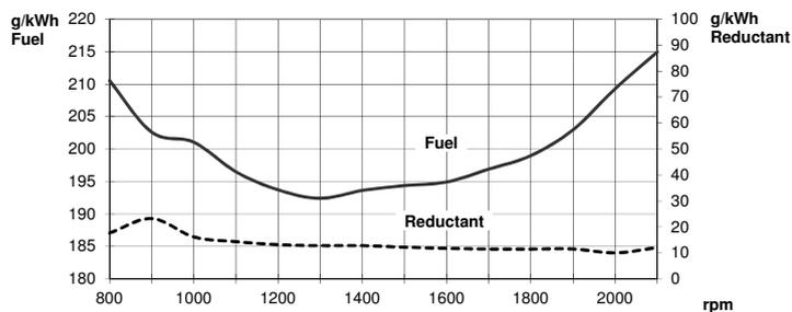
Test conditions Air temperature +25°C. Barometric pressure 100 kPa (750 mmHg). Humidity 30%. Diesel fuel acc. to ECE R 24 Annex 6. Density of fuel 0.840 kg/dm<sup>3</sup>. Viscosity of fuel 3.0 cSt at 40°C. Energy value 42700 kJ/kg. Power test code ISO 3046. Power and fuel values +/-3%.
