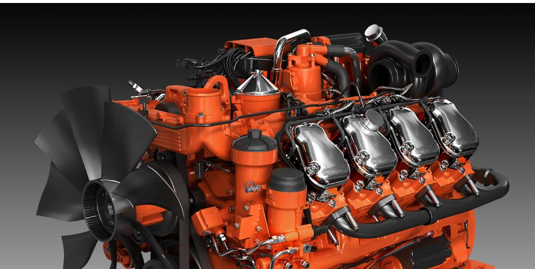
The industrial engines from Scania are based on a robust design with a strength optimised cylinder block containing wet cylinder liners that can easily be exchanged. Individual cylinder heads with 4 valves per cylinder promotes repairability and fuel economy.
